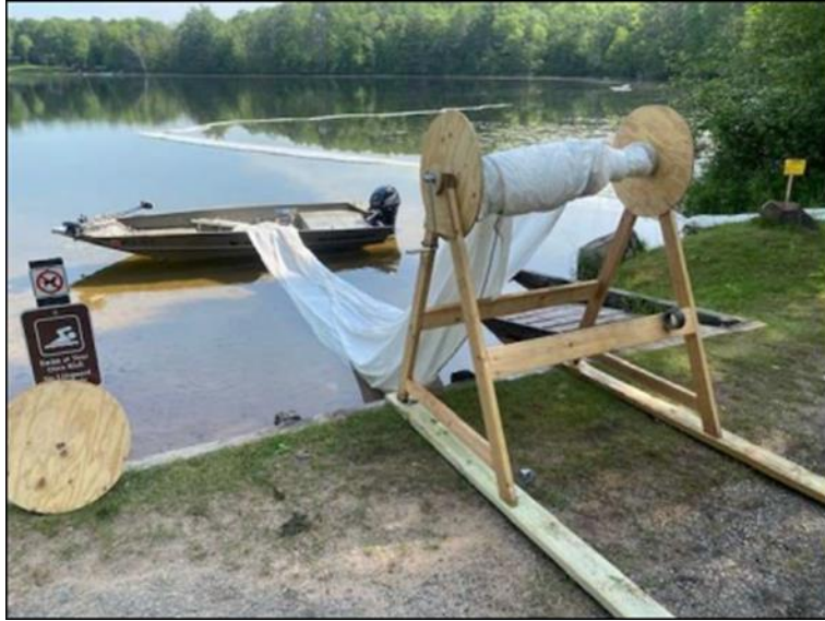
Figure 43: Limno-curtain material on a roll before installation (photo from Marinette Co. LWCD)
