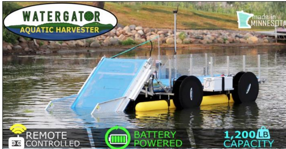
Figure 40: WaterGator remote-controlled aquatic plant harvester ( https://lakeweedharvester.com/watergator/ )
