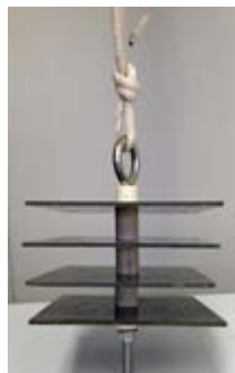
Figure 41. Zebra Mussel Monitoring Equipment: Cinder Blocks and Sampling Plates
