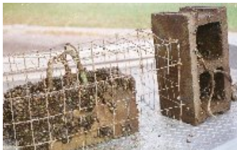
Figure 41. Zebra Mussel Monitoring Equipment: Cinder Blocks and Sampling Plates
