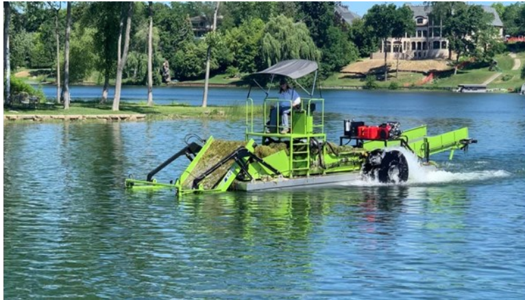
Figure X. Typical mechanical aquatic plant harvester (Photo provided by Inland Lake Harvesters, Inc.)
