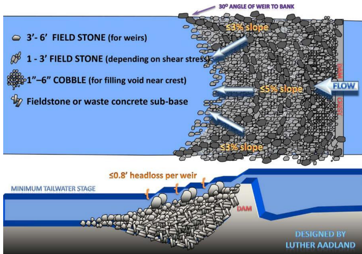
Figure 54. Generalized conceptual design of the Rock Arch Rapids developed by the author.
