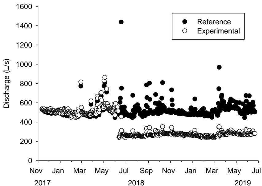
Fig. 2. Time series of mean daily discharge for the Reference and Experimental reaches in Emmons Cr. from mid-November 2017 through mid-June 2019
