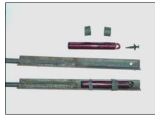
Connected to angle iron welded to re-bar and pounded into stream bottom angled with the flow
