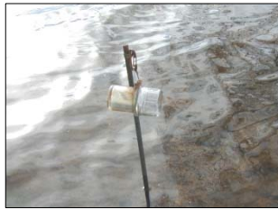
Hobo in capsule attached to fence post or re-bar and pounded into stream bottom
