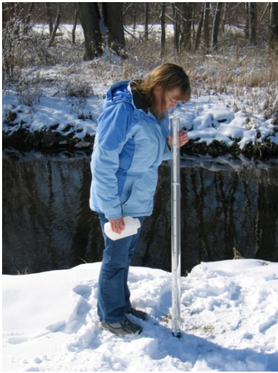
Figure 2: Slowly releasing water until the disk is just visible.
