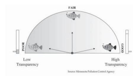
Transparency measurements are affected by both the presence of suspended particles, such as soil particles and microscopic organisms, and by water color, which is caused by certain dissolved substances. Transparency is an easily made measurement that can be correlated with turbidity, although the two measurements are not directly comparable.
