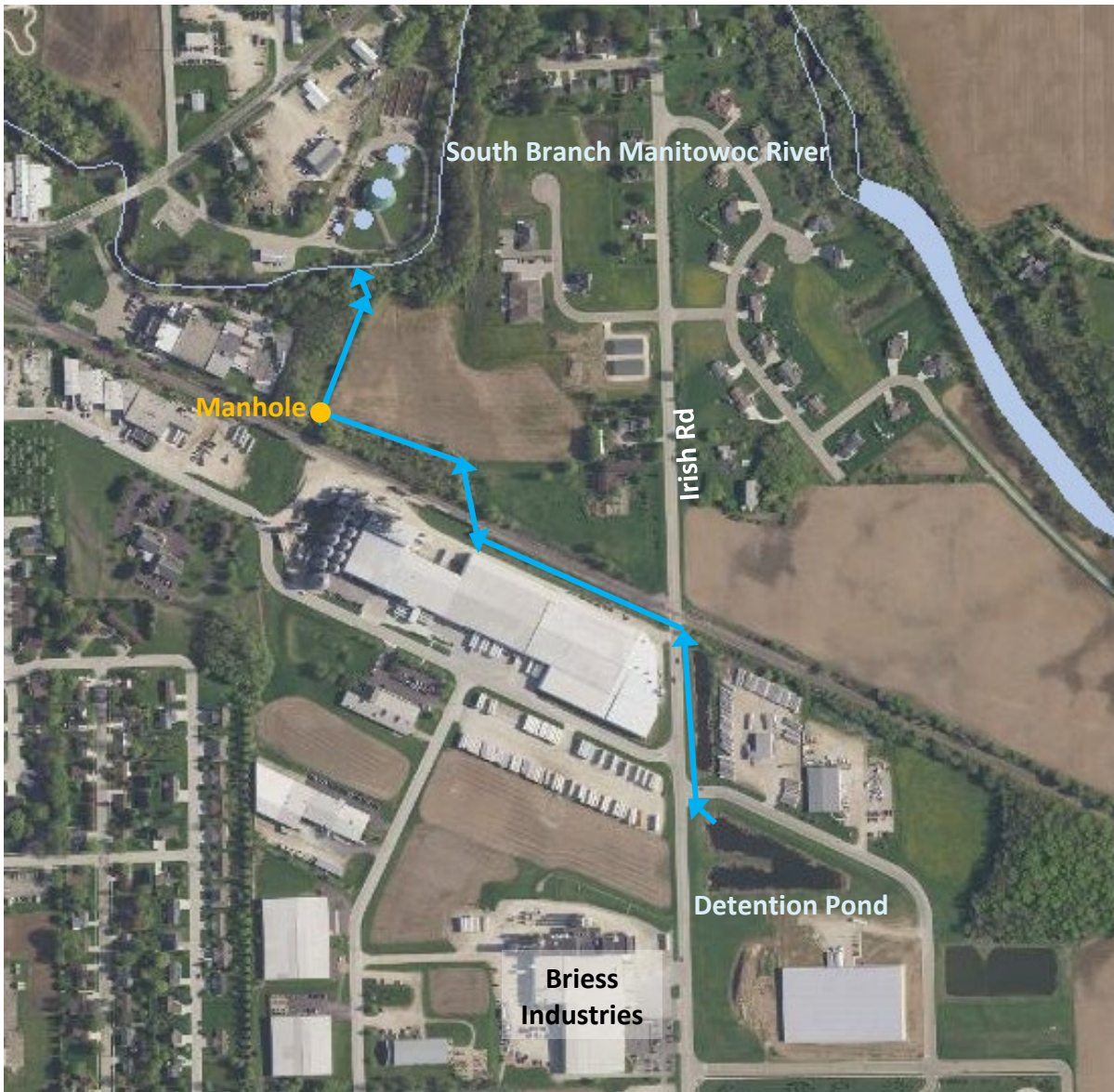
Map 1. Flow path from the detention pond receiving effluent from Briess Industries to the South Branch Manitowoc River.
