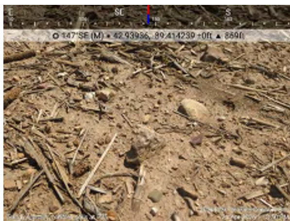
Photo #42 Gravelly/cobbley soils at P05
