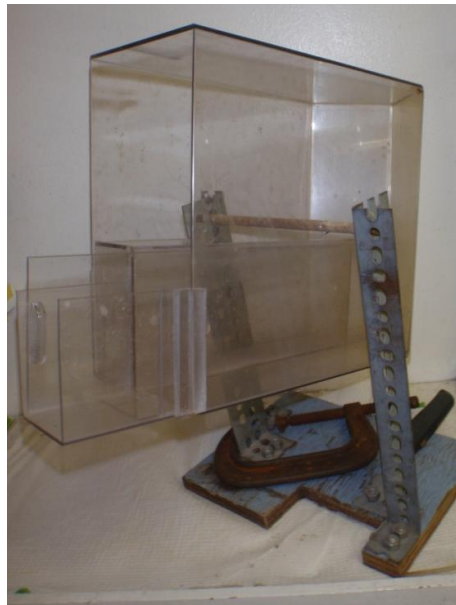
Figure 1. Photograph of LSRI's Benthic Invertebrate Subsampler, which is modeled after the Folsom Plankton Splitter. The Benthic Invertebrate Subsampler has a rectangular-shaped box with a V-shaped bottom and spouts attached to the sampler to facilitate removal of the subsample.
