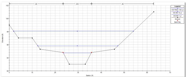
Figure 1 – Sample proposed cross section modeled showing 1 yr, 10 yr, and 100 yr water elevations
