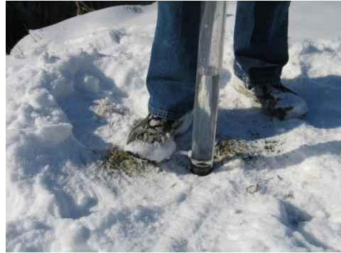
Figure 2: Slowly releasing water until the disk is just visible.
