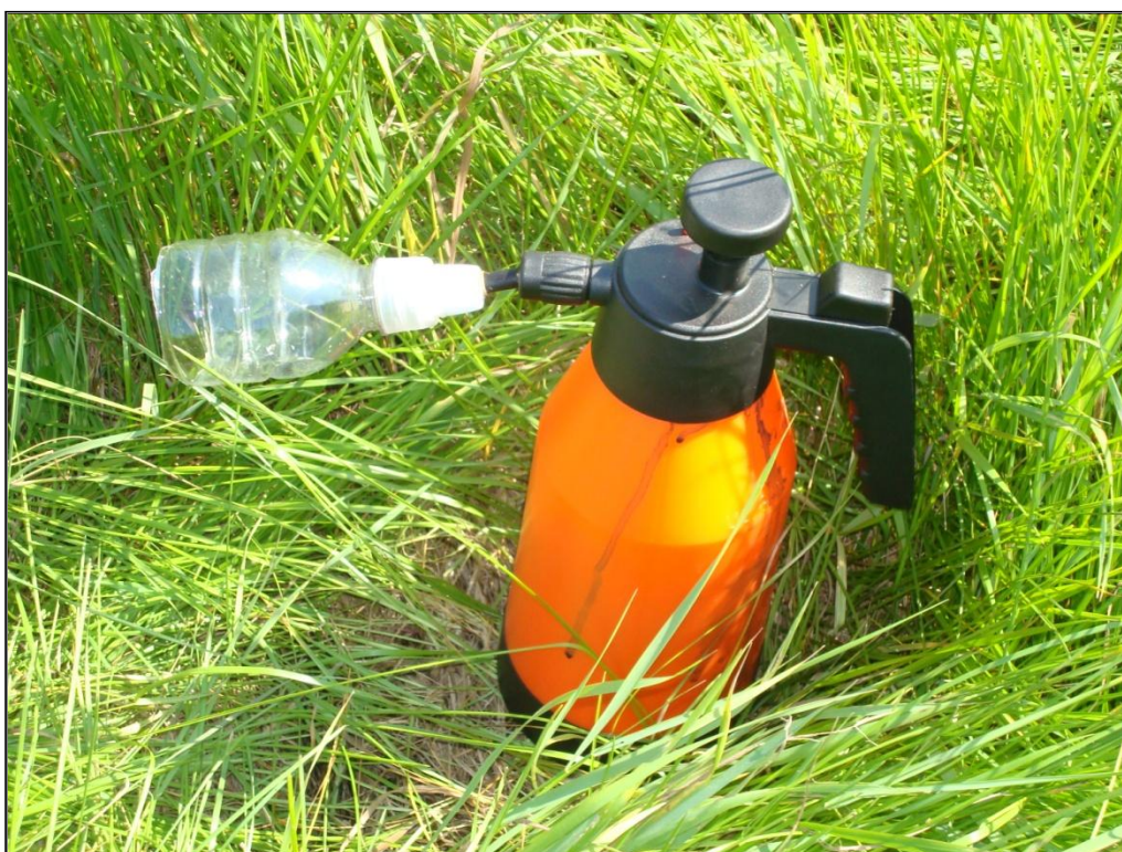
Figure 10: Small capacity compression sprayer modified with a drip/drift guard.
