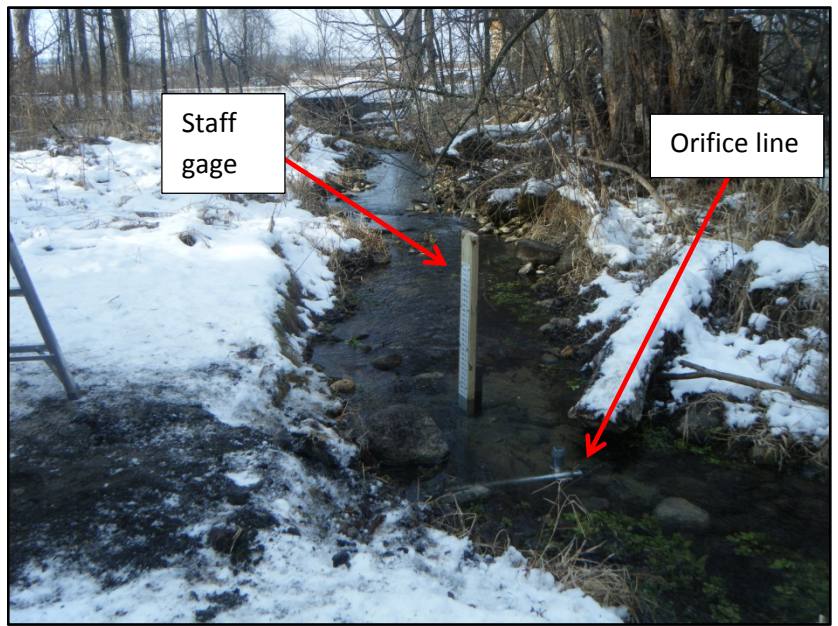
Staff gage and orifice line in creek (looking downstream to the east). Gage house is out of view to the left.
