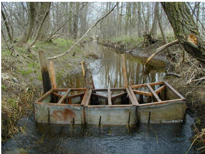
Figure 4. Three side-by-side fish larvae trap assembly deployed at Ulao Creek station UC1. Note incised channel morphology.
