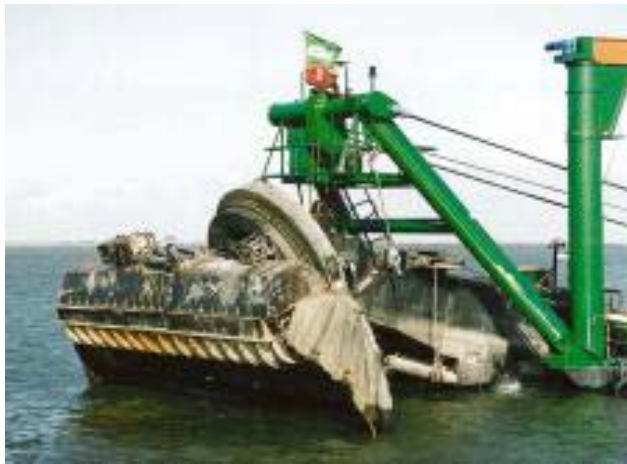
Hydraulic Horizontal Auger Dredge Source: D.C. Roukema, J. Driebergen, and A.G. Fase
