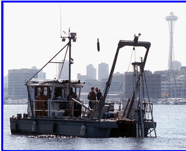
Vibracore Sampling Source: ThermoRetec
