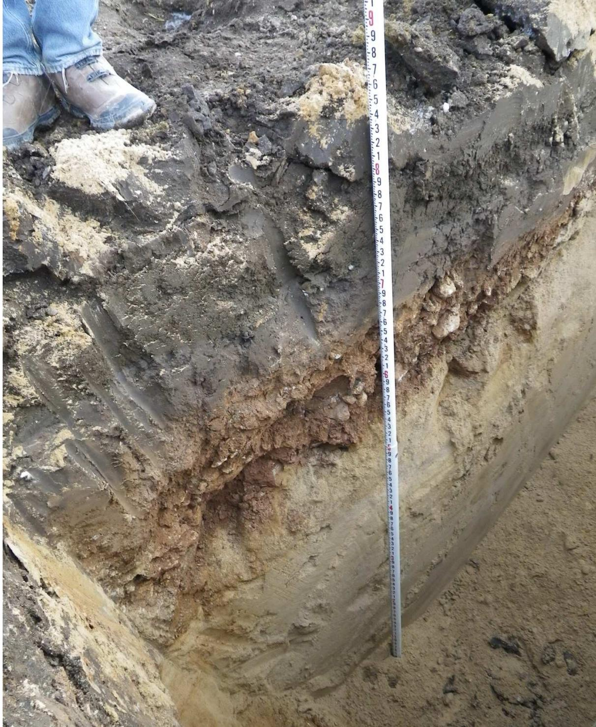
Soil Depth Adequate for Separation to Bedrock and Water Table
