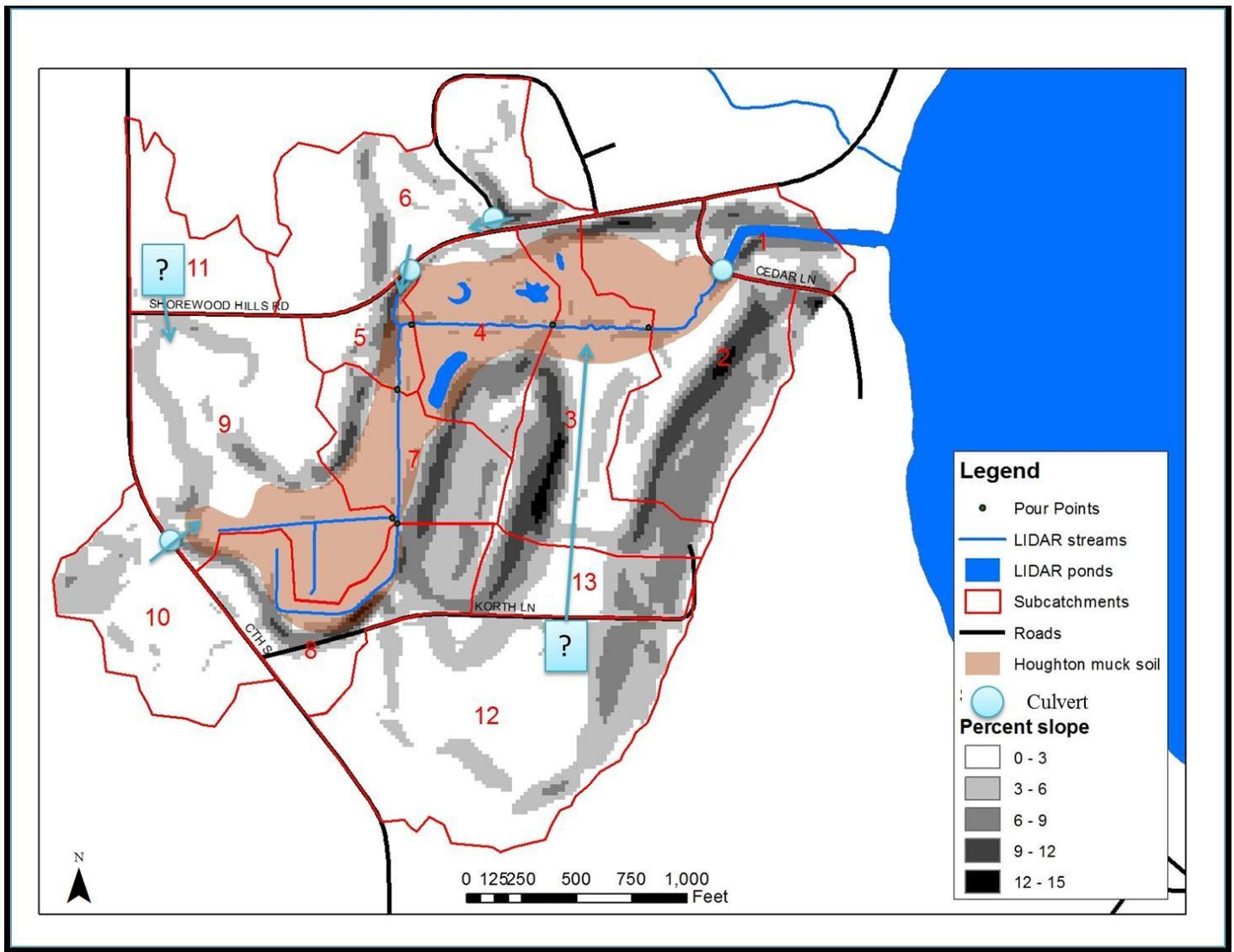
**FIGURE 2.30 SUBWATERSHEDS DELINEATED IN GIS. NUMBERS 11, 12, AND 13 DO NOT CONTRIBUTE RUNOFF TO DITCH UNDER NORMAL CONDITIONS.**
