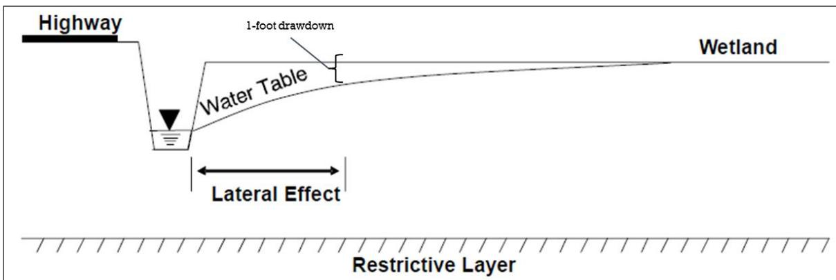
FIGURE 2.23 LATERAL EFFECT ILLUSTRATION. LATERAL EFFECT IS THE DISTANCE FROM THE DITCH THAT IS ADEQUATELY DRAINED WITHIN SOME CRITICAL PERIOD (ADAPTED FROM SKAGGS ET AL. 2005).
