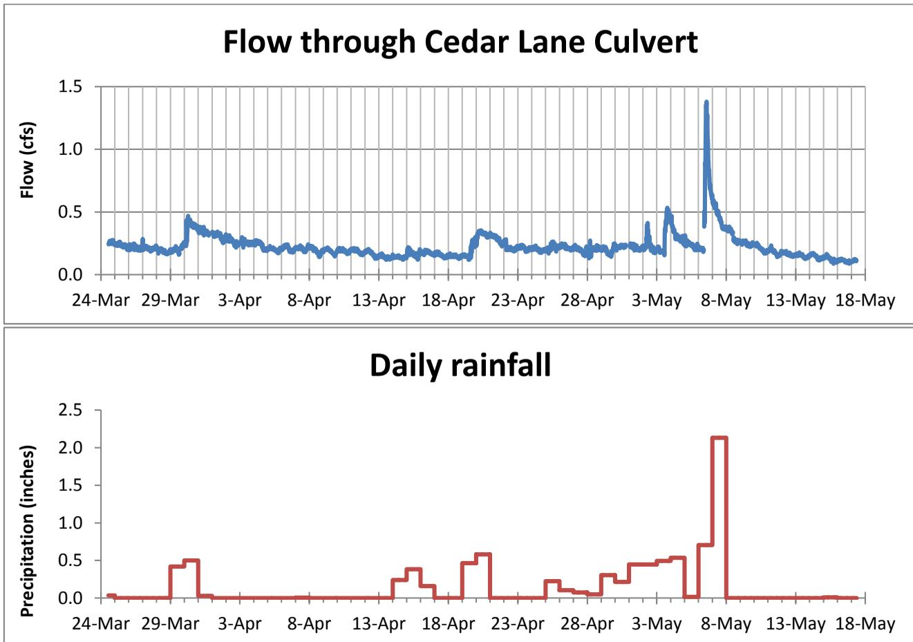
FIGURE 2.6 EXAMPLE OF CONTINUOUS FLOW DATA COLLECTED AT CEDAR LANE CULVERT.
