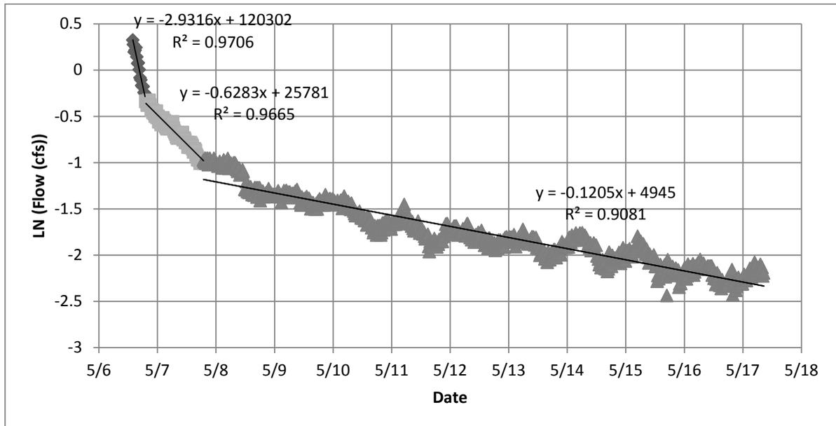
**FIGURE 2.8 HYDROGRAPH RECESSON AFTER 1.77 INCH STORM, PLOTTED ON LOG SCALE. THE CHANGE IN SLOPE INDICATE A SHIFT FROM QUICKFLOW TO BASEFLOW.**
