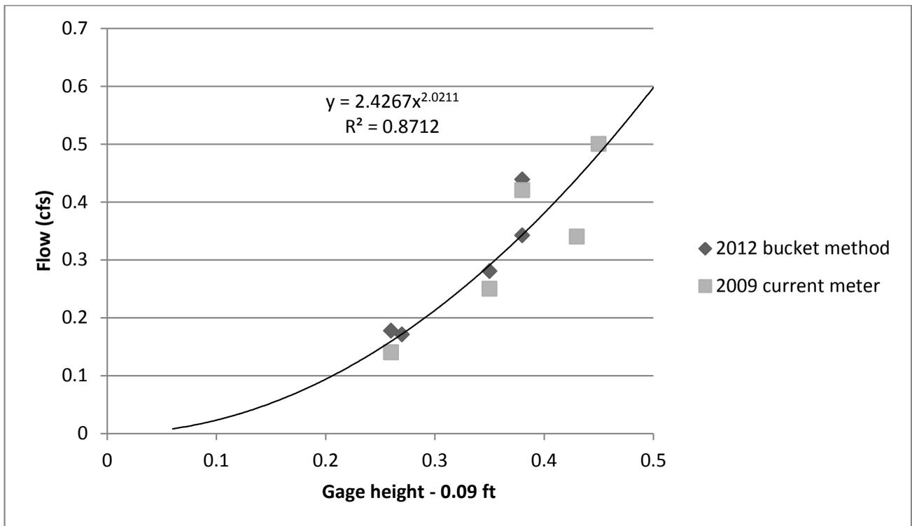
FIGURE C.5 RATING CURVE FOR THE DITCH AT CEDAR LANE CULVERT.  $Q=2.4267(G-0.09)^{2.0211}$
