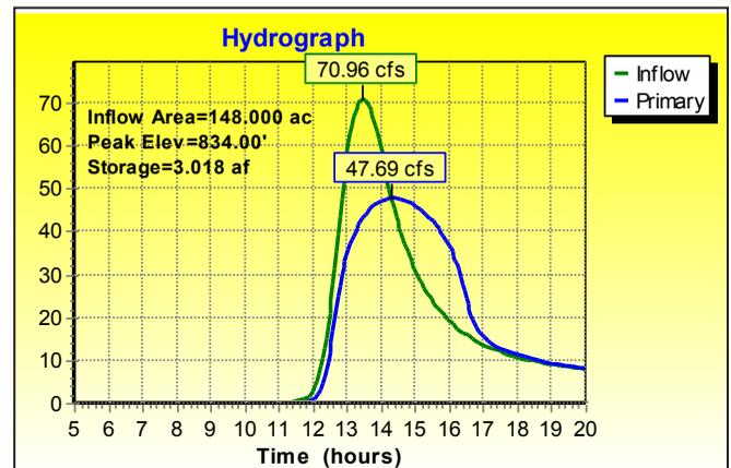
FIGURE 2.25 PEAK FLOW SUFFICIENT TO OVERTOP CEDAR LANE (ELEVATION <834).
