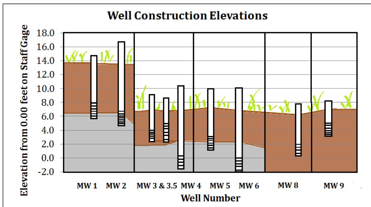
FIGURE H.1 WELL CONSTRUCTION DIAGRAM OF THE WELLS LOCATED IN THE WATERSHED. GREY REPRESENTS THE SILTY-CLAY LAYER AND BROWN REPRESENTS THE HOUGHTON MUCK. ALL ELEVATIONS HAVE BEEN SURVEYED TO 0.00 FEET ON THE STAFF GAGE.
