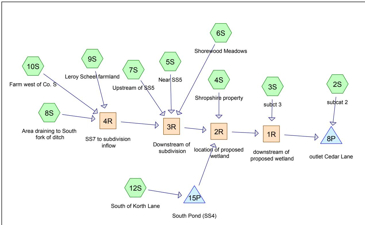
FIGURE E.1 DIAGRAM OF CATCHMENTS (S), REACHES (R), AND PONDS OR OUTLETS (P) IN HYDROCAD MODEL.
