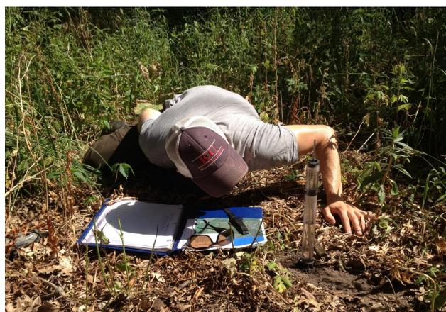
**FIGURE C.3 SOIL INFILTRATION TEST. CONDUCTED BY MIKE DRAPER. PHOTO CREDIT: STEVE NEARY, 6.15.12**
