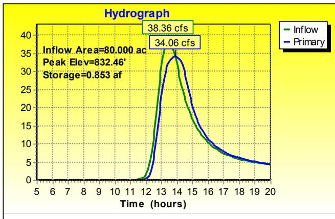
FIGURE 2.24 PEAK FLOW SUFFICIENT TO SUBMERGE CEDAR LANE CULVERT (ELEVATION 832.26).
