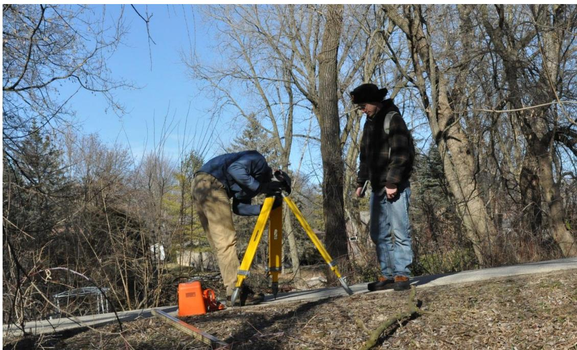
**FIGURE C.4 CONDUCTING A LANDSCAPE SURVEY TO GAIN ACCURATE ELEVATION DATA FOR MONITORING WELLS AND THE STAGE RECORDER. PICTURED ARE TOM BENEKE AND JOSH BOHNERT. PHOTO CREDIT: STEVE NEARY, 3.9.12**
