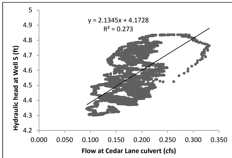
**FIGURE 2.19 POOR CORRELATION BETWEEN WATER TABLE AND GROUNDWATER DISCHARGE TO DITCH.**
