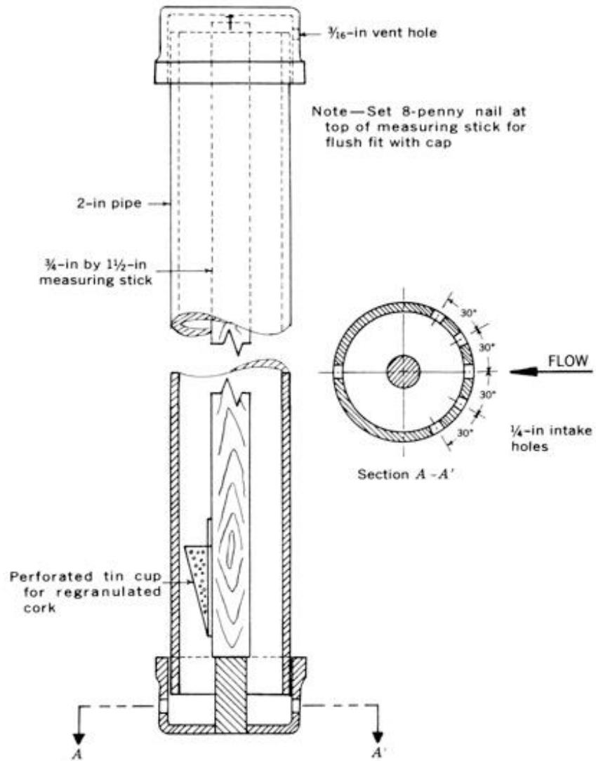
FIGURE C.7 CREST STAGE GAGE DIAGRAM. SOURCE: U.S. GEOLOGICAL SURVEY (USGS.GOV).
