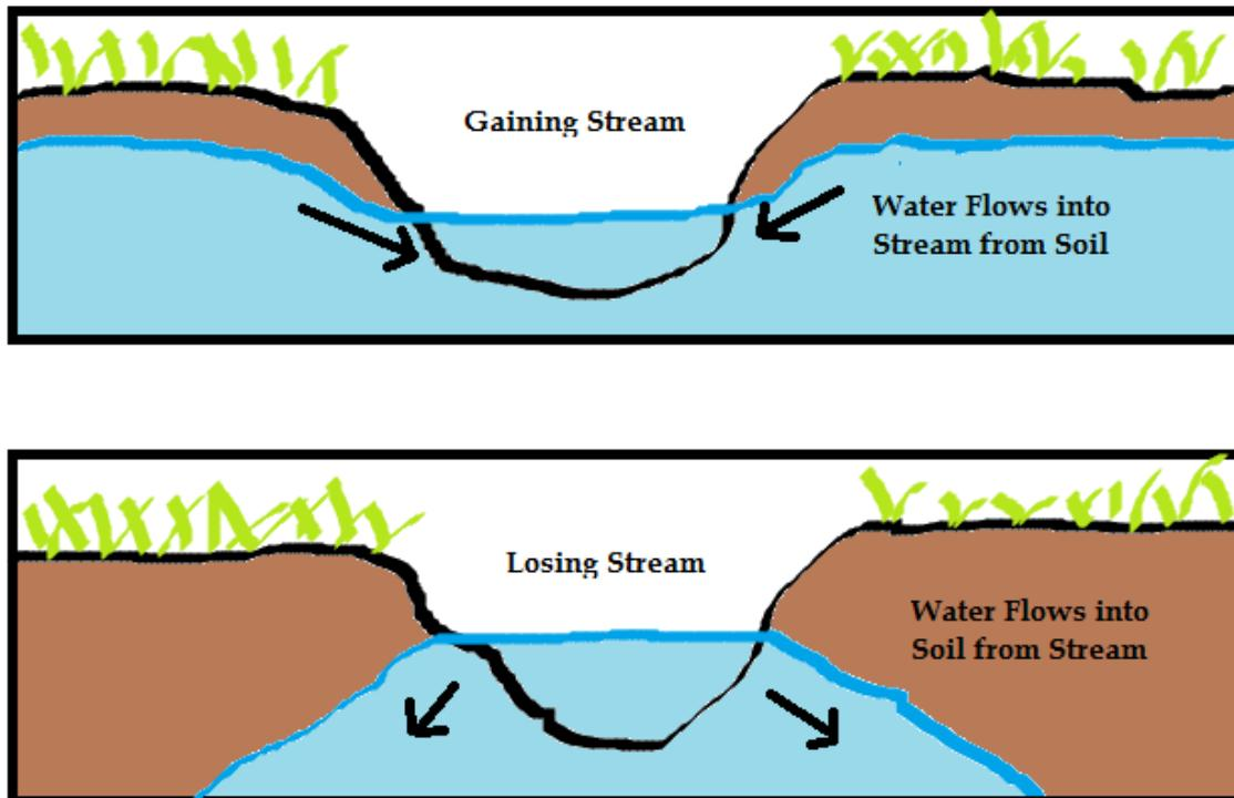
**FIGURE 2.21 GAINING STREAMS HAVE HIGHER WATER TABLE ELEVATIONS WITHIN WELLS THAN STREAM STAGE ELEVATIONS. IN THIS INSTANCE, WATER FLOWS FROM THE GROUNDWATER INTO THE STREAM. LOSING STREAMS HAVE FLOW OUT OF THE STREAM INTO THE GROUND. WATER TABLE ELEVATIONS LOWER THAN STREAM STAGE ELEVATIONS INDICATE LOSING REACHES.**
